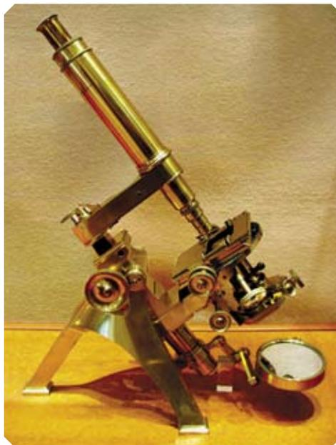
A microscope is an instrument for viewing objects that are too small to be seen by the unaided eye. Today, there are electron microscopes, using magnetic fields and electron rays instead of lenses and light, making it possible to see even atoms.
