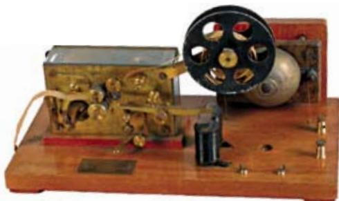
Morse code uses short and long elements (known as “dots” and “dashes”) to transmit information. Originally created for an electric telegraph, it was often used for early radio communication.
